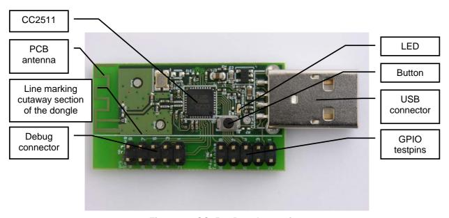
Figure 11: CC2511 Dongle top view
